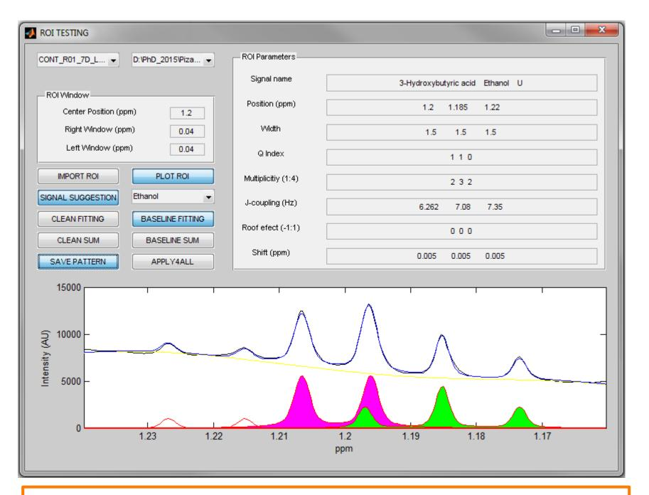
The 'BASELINE FITTING' mode allows deconvolving targeted signals in ROIs where baseline or broad signals are affecting the final shape of the region; it will take more computation time but is the optimal solution in those cases.
