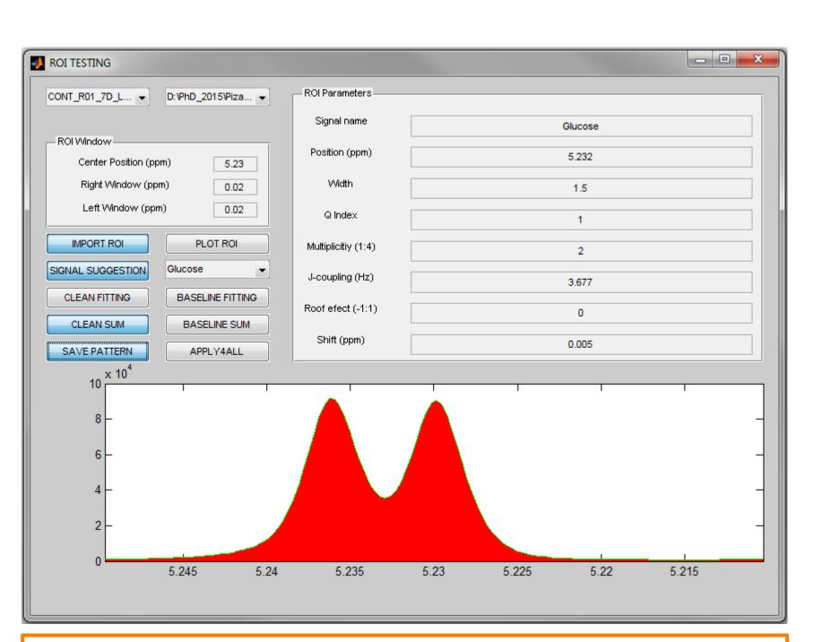
•The 'CLEAN SUM' mode is very useful for those ROIs that contain isolated and pure (without any baseline) signals because the computation time is severely reduced while the quantification remains accurate.
