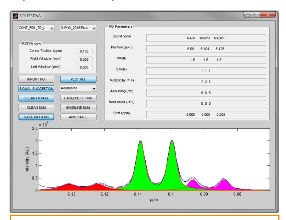
•The 'CLEAN FITTING' mode is able to quantify accurately overlapping signals in ROIs where neither baseline nor broad signals are affecting.
